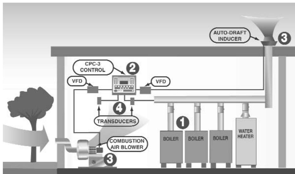
The heaters will be disrupted for 1 minute if at any time the draft cannot be maintained within the times and tolerances of the software. After this restart delay the CPC-3 will once again try to reach the system set points. If successful, the system will sequence normally. If not successful, the CPC-3 will lock out the heaters until it is manually reset. Up to 5 fault codes will be stored memory.
