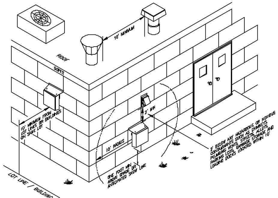
On wall installations, if possible, terminate the Intake Hood on a wall that does not face the direction of prevailing winds. This will diminish the possibility of wind infiltration.
