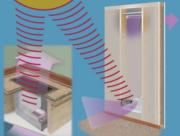
ASLL Level-To-Level Transfer Fan
