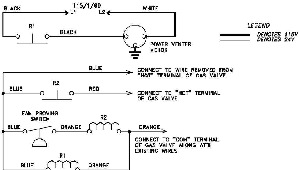
The diagrams below represent common ways in which the HS-3, HS-4, HS-5 Power Venters are interlocked to 24V controlled appliances. Variations of these diagrams are acceptable as long as the Fan Proving Switch isolation circuit is wired to disable the gas valve if a venting malfunction should occur.
