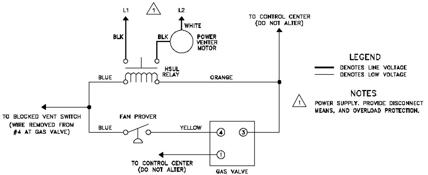
**HST SERIES CONNECTED TO AN R8184G WITH THE APPLIANCE
