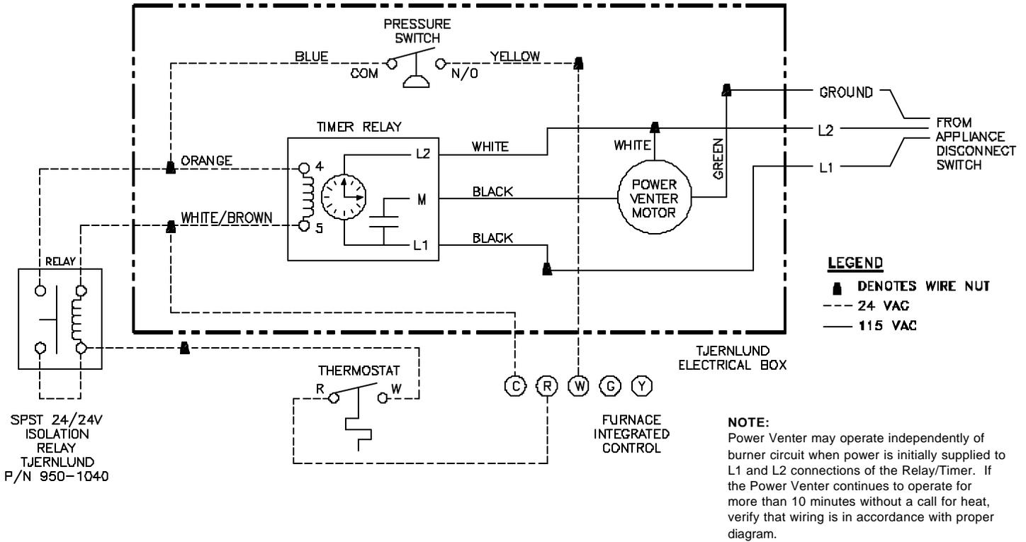
**HS115 SERIES CONNECTED TO ANY 115V BURNER MOTOR OR GAS VALVE
