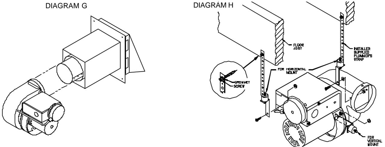
4. Verify required vent pipe diameter from "Power Venter Selection" on Page 1. Verify that a full sized barometric control has been installed on appliances not equipped with a draft hood or draft diverter.
