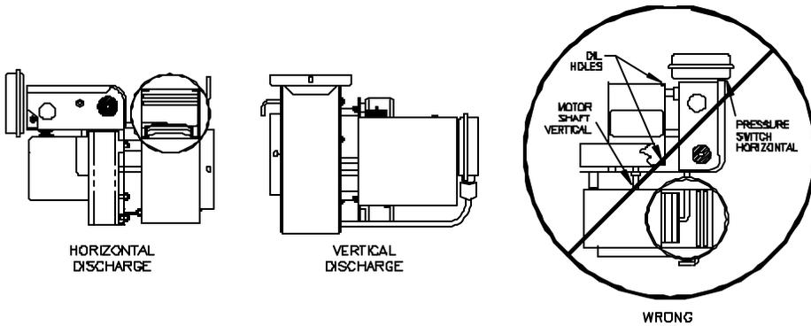
3. The Power Venter housing is single wall. A 15.2CM (6") clearance to combustibles must be maintained for gas and 45.7 CM (18") clearance for oil applications, (See Diagram C).
