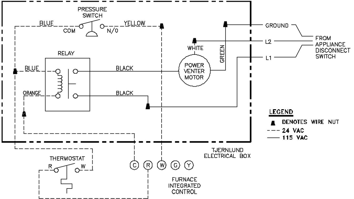
**HST SERIES CONNECTED WITH THERMOSTAT ON SINGLE ZONE 24V GAS EQUIPMENT**
