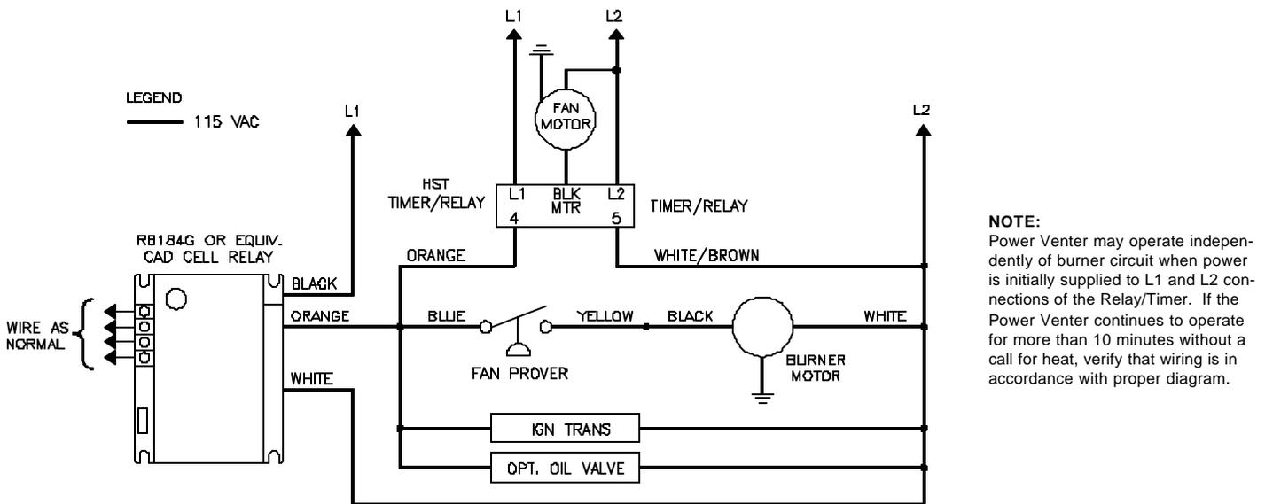
NOTES: The Power Venter is usually interlocked with the primary control of the appliance. Wire all other furnace/boiler controls as normally done when conventional venting before continuing. Disconnect power from the appliance before attempting to interlock the Power Venter.
