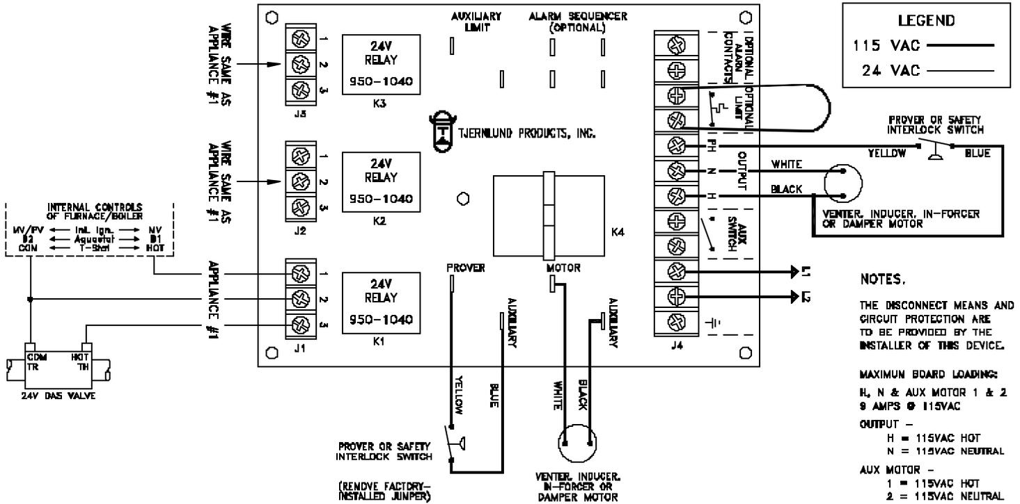
MAC-3 CIRCUIT BOARD WIRING SCHEMATIC
