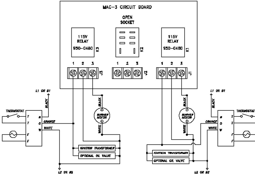
MAC-3 WIRED WITH UP TO FIVE 24V GAS BURNERS AND ONE POWER VENTER, DRAFT INDUCER OR IN-FORCER
