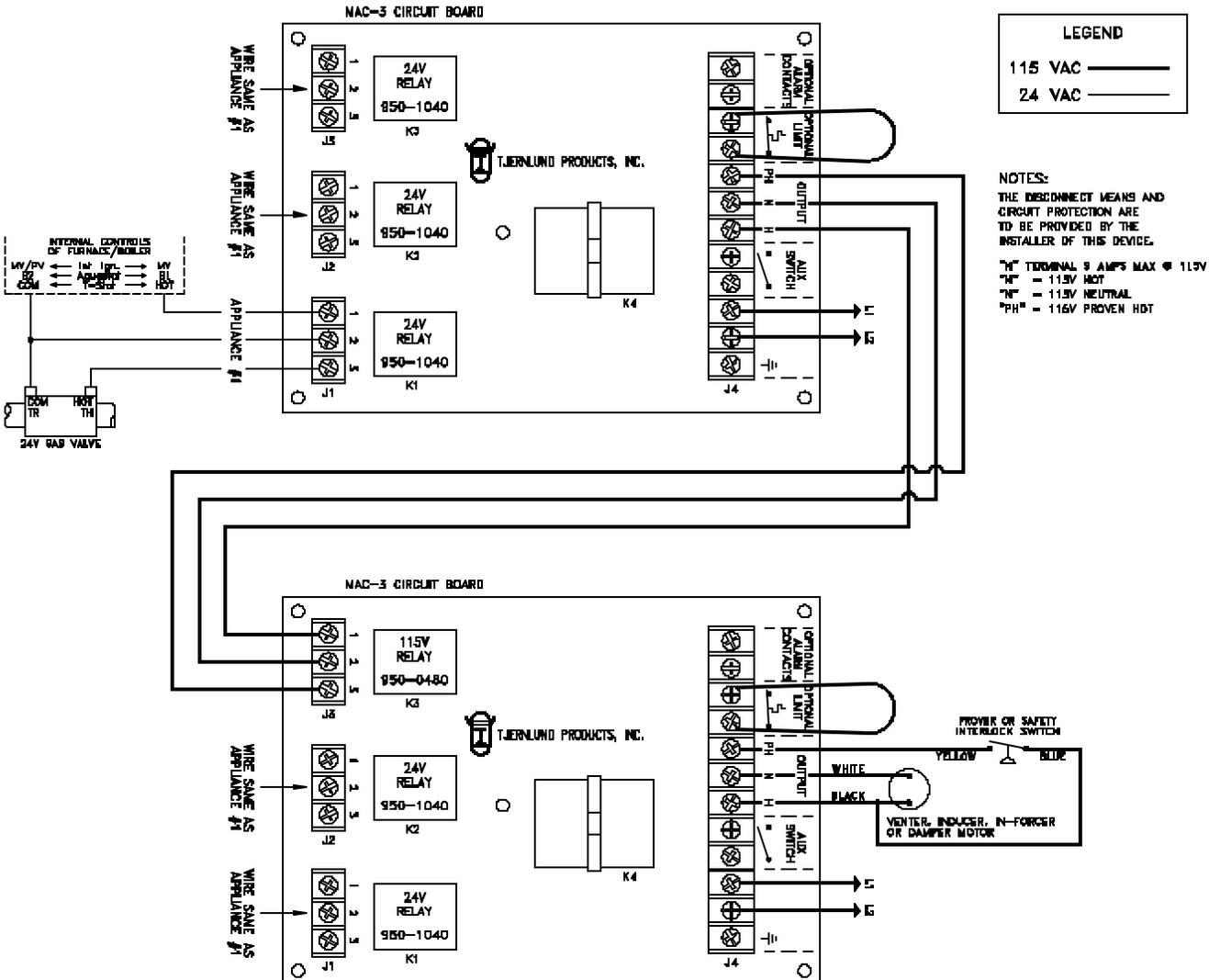
MAC-3 WIRED WITH A POWER VENTER OR DRAFT INDUCER AND A COMMERCIAL IN-FORCER
