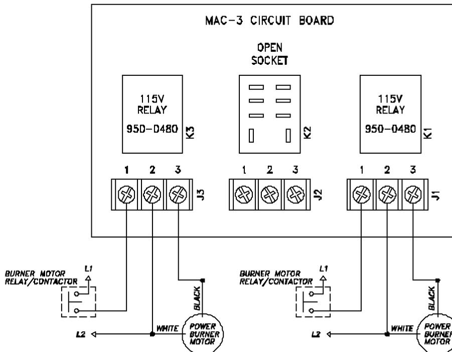
MAC-3 WIRED WITH UP TO THREE OIL BURNERS WITH R8184G CONTROLS - BURNER MOTOR LESS THAN 7 AMPS
