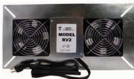
The RV2 Radon Ventilator exhausts radon and other harmful soil gases and allows fresh outdoor air to replace them. At 220 CFM, the RV2 ventilates a 20' x 40' x 3' crawl space over 5 times per hour while using only 40 watts. Simply mount the unit against a vent opening with the included hardware and plug it in. For even greater results multiple units can be installed. Run it continuously or with a plug-in timer. Also helps reduce crawl space humidity.
