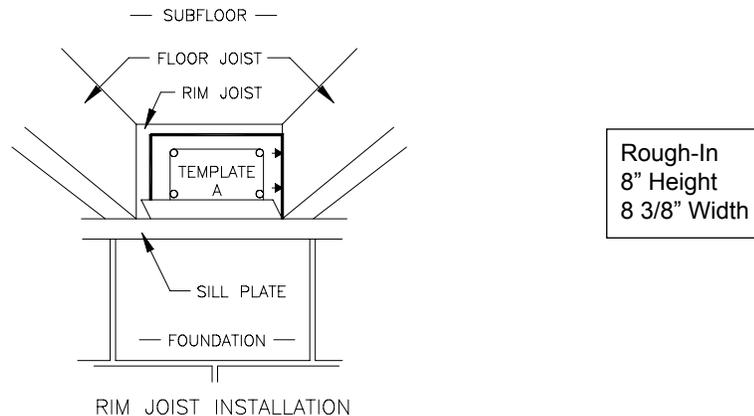
2. Using 1/2" bit, drill pilot holes noted on each side of the template from inside through rim-joist, wall board, siding, etc., keeping drill bit perpendicular to the wall. 1/2" bit must be long enough to penetrate through exterior.
