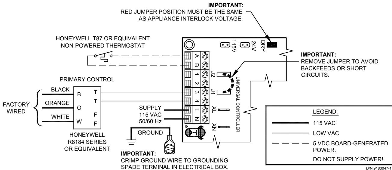
1. **IMPORTANT:** Remove J1 & J2 Call Jumper on UC1 to avoid backfeeds or short circuits.
