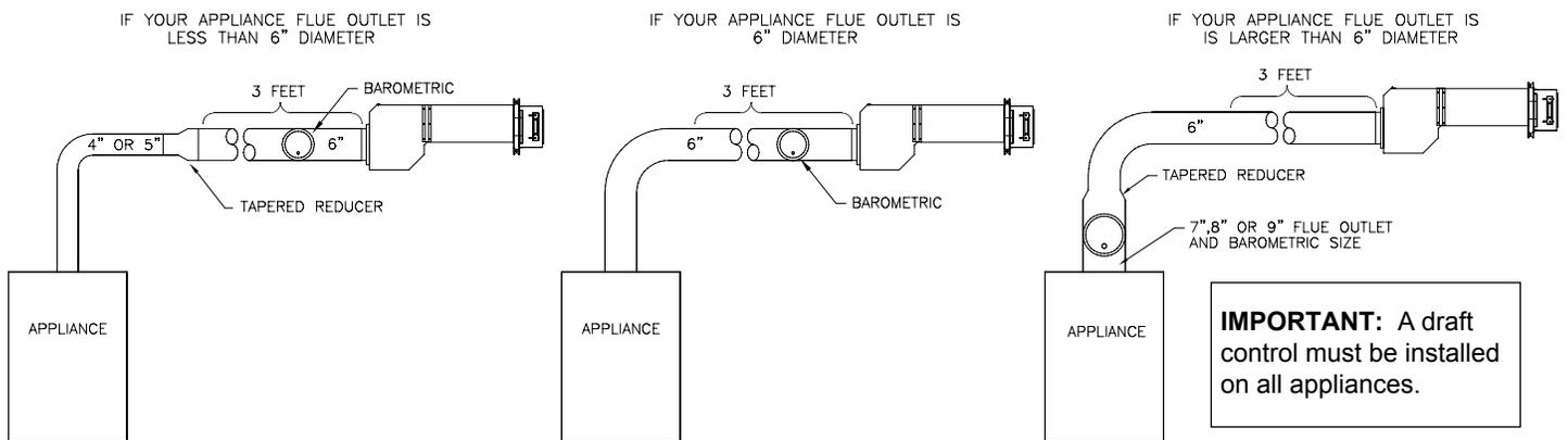
**IMPORTANT:** A draft control must be installed on all appliances.
