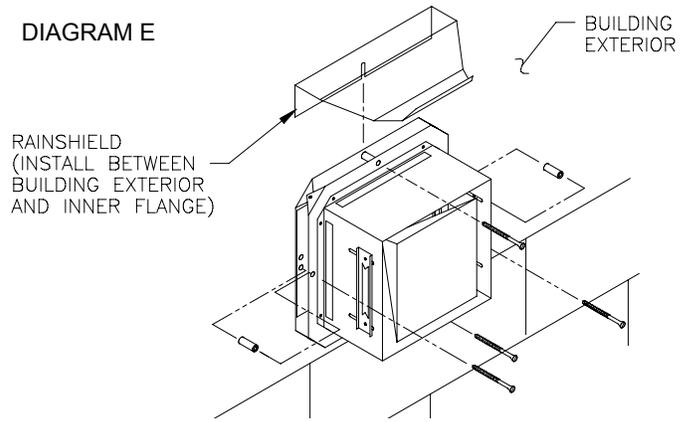
**NOTE:** For mounting on vinyl or lap siding a wood frame with 1" x 1 1/2" on the sides and top and 1" x 2" material on bottom can be utilized on exterior wall. This will provide a flush mounting surface for the hood and a nicely finished look with "J" channel when siding. Inside of frame opening should be 8 3/8" wide by 8" high.
