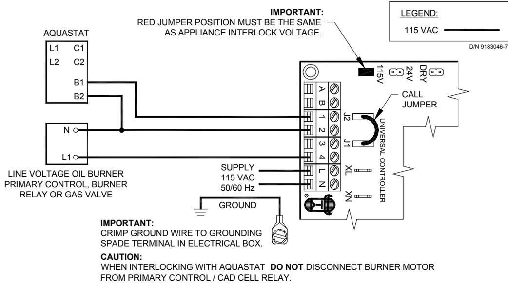
1. Disconnect B1 from L1 of oil burner primary control, burner relay or hot of gas valve and reconnect to #1 on UC1 terminal block.
