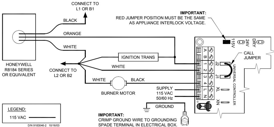
1. Separate the Black burner motor wire from the Orange wire of R8184 Primary Control.
