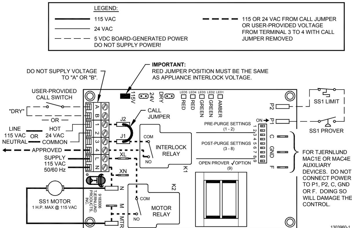
**WARNING:** Disconnect power supply from the SS1C and heating equipment when making wiring connections and servicing the SS1C. Failure to do so may result in personal injury and/or equipment damage. LED #5 (RED) should be off with power removed.
