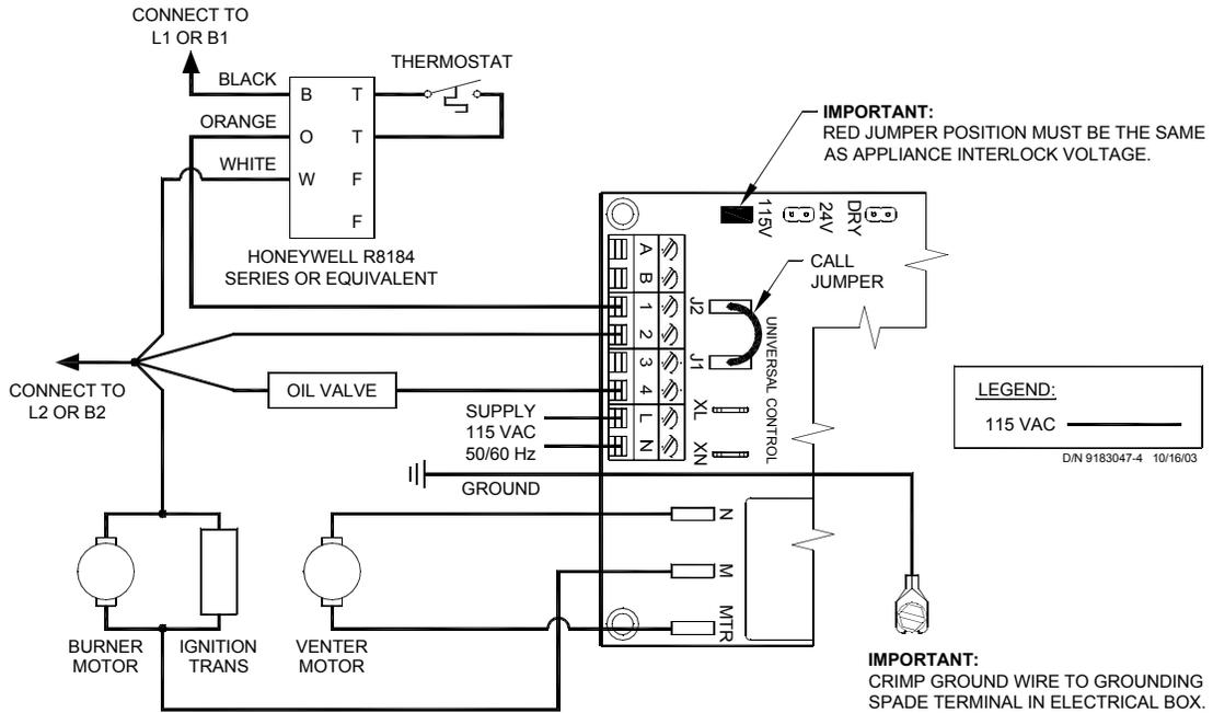
1. Separate the burner motor wire and ignition transformer from the Orange wire of R8184.
