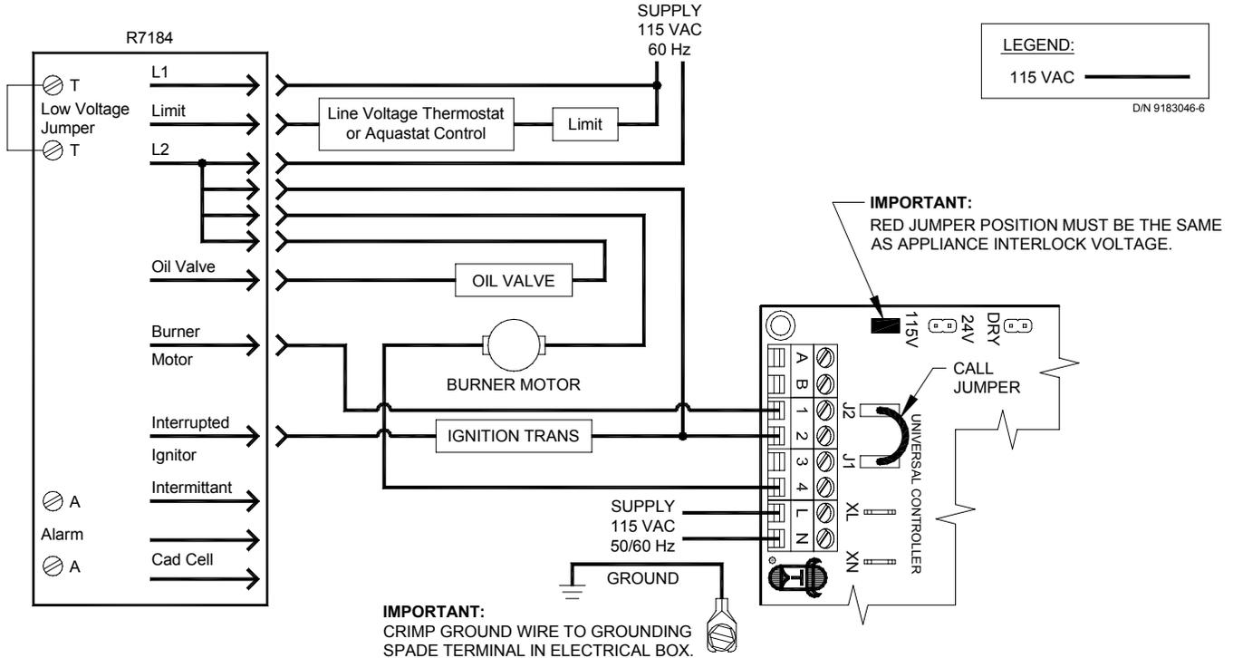
1. Disconnect burner motor wire off the R7184.
