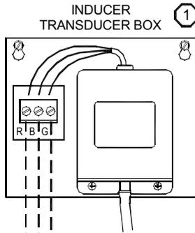
Route transducer wiring in metal conduit or use Belden Shield Cable #9939 or equivalent. Make sure the transducer wiring does not contain or cross line voltage wiring or undesired transducer performance may result.
