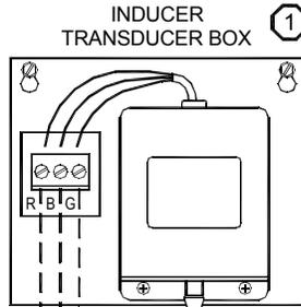
Route transducer wiring in metal conduit or use Belden Shield Cable #9939 or equivalent. Make sure the transducer wiring does not contain or cross line voltage wiring or undesired transducer performance may result.
